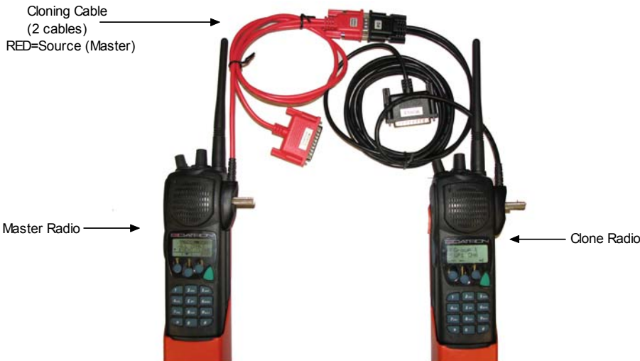
Fig. 8: Cloning Cable Connections
